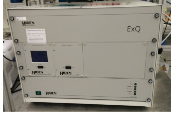
Product analysis in the exhaust stream of the experimnt. Here, the mass spectrometer at P65. Alternatively an FTIR gas analyser will be available.
