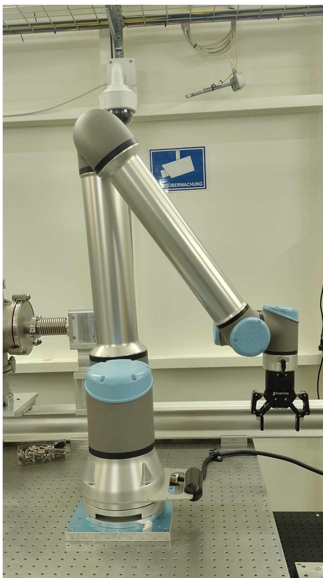
Universal robots UR10e at beamline P65, will be used as sample changer for automated and remote controlled in-situ experiments.
